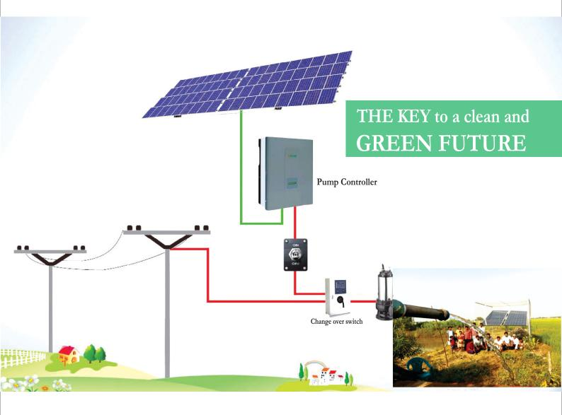
Solar Pumping Systems are extremely useful for running AC pumps for agriculture, domestic or industrial applications. These systems consist of a pump controller which draws power from solar panels and run the pump through a variable speed drive controller.
